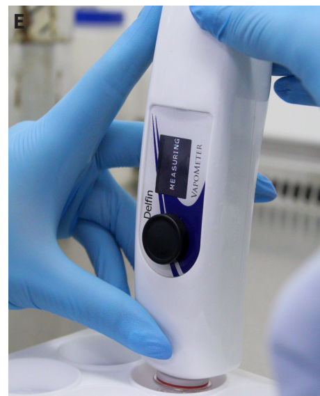
Above: (D.) Bioengineered full thickness human skin model (sample prepared for histology and stained with H&E). (E.) Compatibility with instrumentation used in the clinic (example shows measurement of transepidermal water loss).
