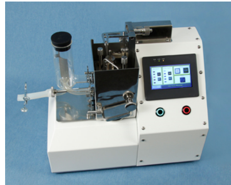
Precision-cut slices (250 or 500 µm thickness) are generated using a Krumdieck tissue slicer
