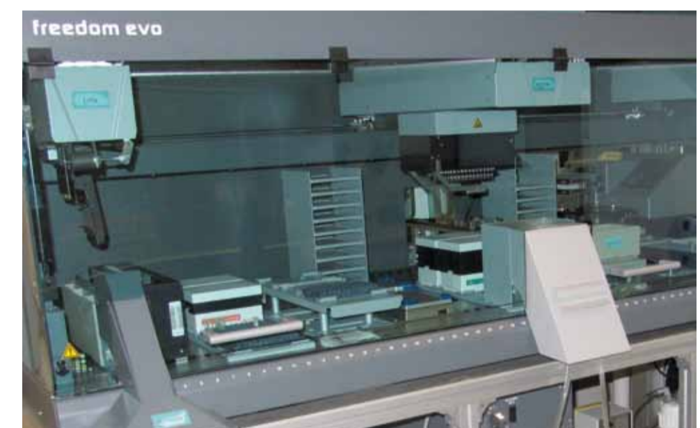
Figure 2: Freedom EVO 200 with 8-channel Liquid Handling Arm, MCA 96 and integrated gripper, cooling carrier, shaker, carousel and incubator (StoreX 110, LiCONiC)
